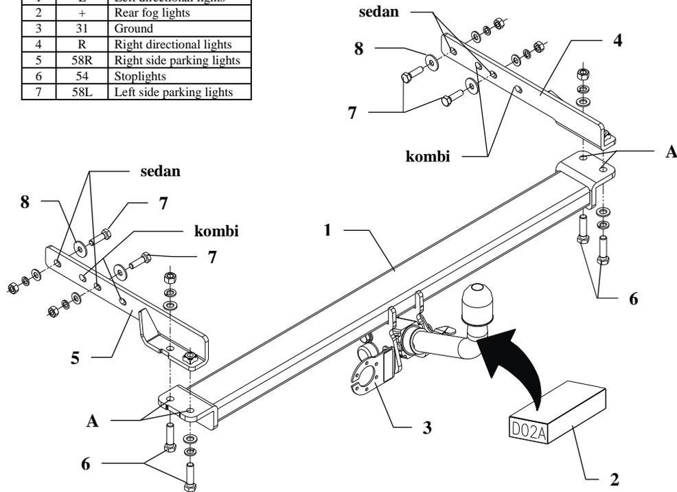
This towbar is designed to assembly in following car:
